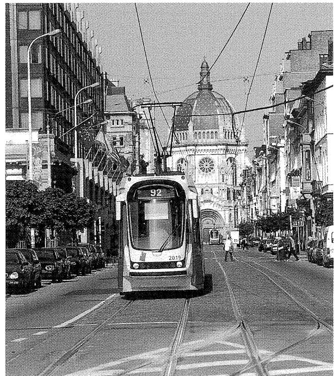
FIGURE 13-22 Brussels, Belgium, subway and tram lines. European cities such as Brussels have invested substantially to improve public transportation in recent years. Brussels provides a good example of a public transport system that integrates heavy rail (Métro Lines 1 and 2) with light rail (trams). Trams initially used Métro tunnels, but the tunnels were large enough to convert to Métro-rail lines as funds became available. The photograph shows a line 92 tram on the Rue Royale.
